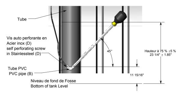
Passez le cable de la flotte à travers le tube (B) et serrez la vis (D) Pass the float cable through the PVC pipe (B) and tighten the screw (D)
